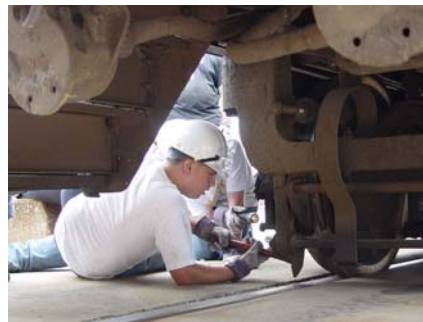
Replacing a brake shoe at Steamtown
